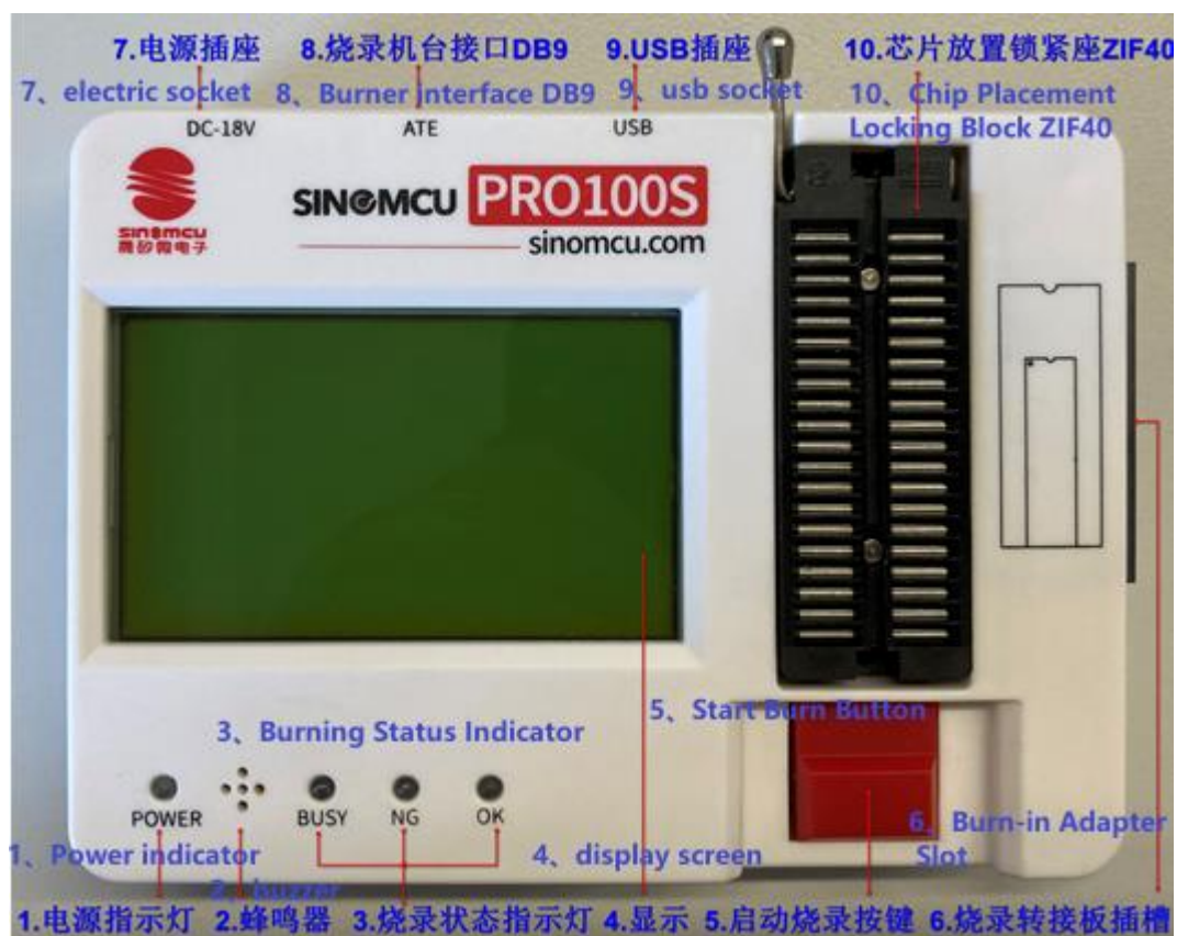
Figure 2-1 Names of hardware interfaces
