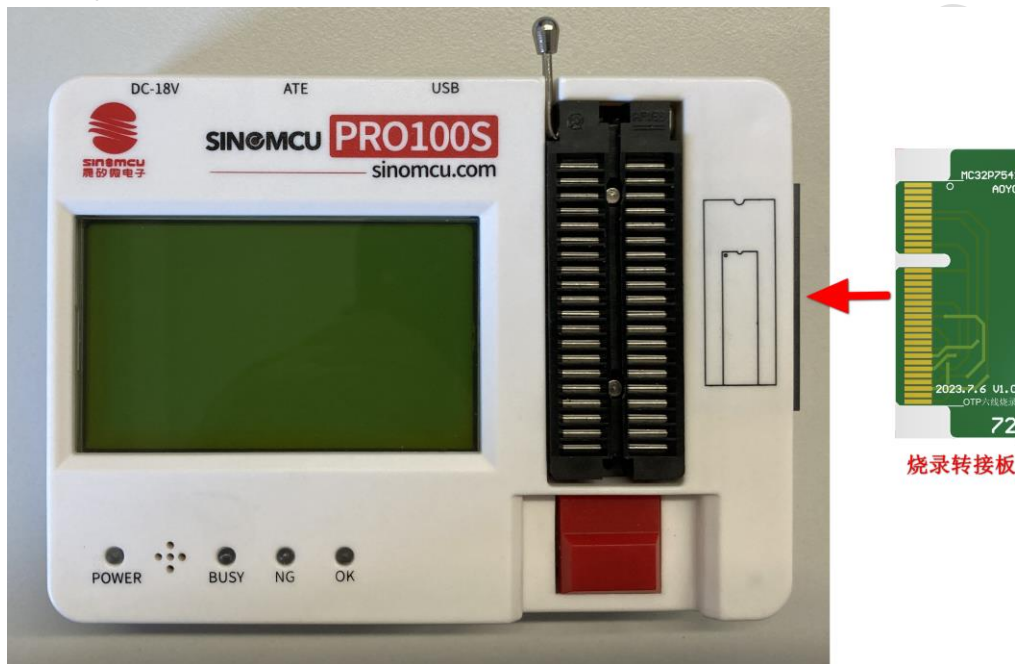
Figure 2-3 Standard burn-in adapter board connected to burner
