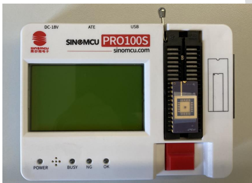
Figure 2-6 Placing the Chip
